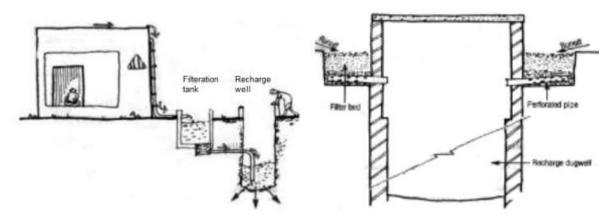
Fig. 6 Simple diagrams showing roof-top rainwater harvesting and surface run-off harvesting
