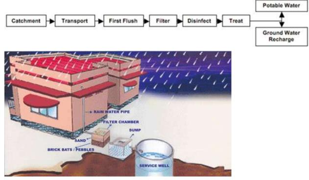
Fig. 10 Rainwater Harvesting at individual level
