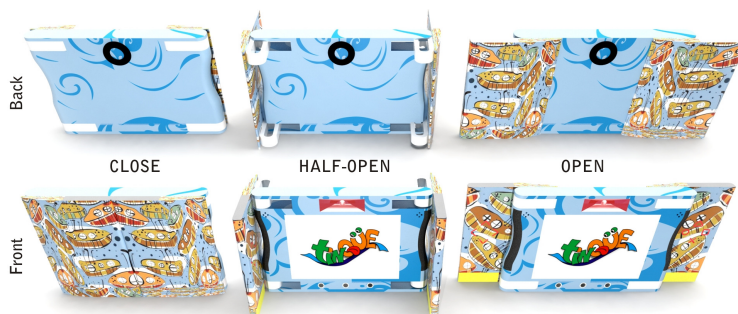
Figure.5 explain open/close system of min projector
