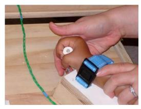
Figure.9 Wrist Extension Racecar Controller
