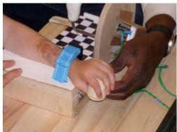
Figure.7 Wrist Extension Racecar Controller
