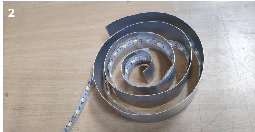
The strip is wrapped around a cylindrical object and taken out to create a spiral surface.
