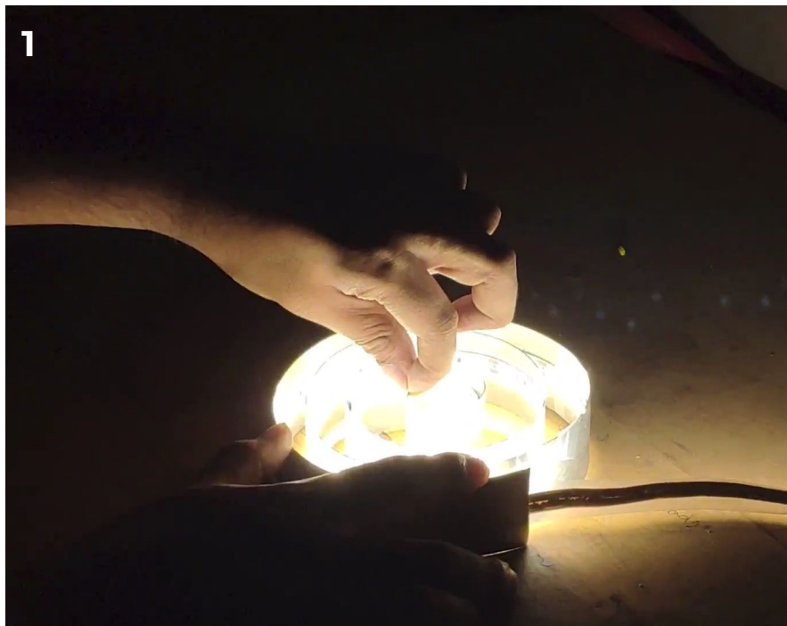
When in the closed stage, the surfaces block the light from spreading sideways and create a unidirectional lamp like a spotlight.
