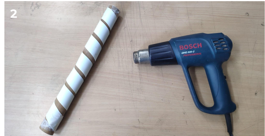
The strip is wrapped around a cylindrical object and hot air is blown over it to retain the shape.
