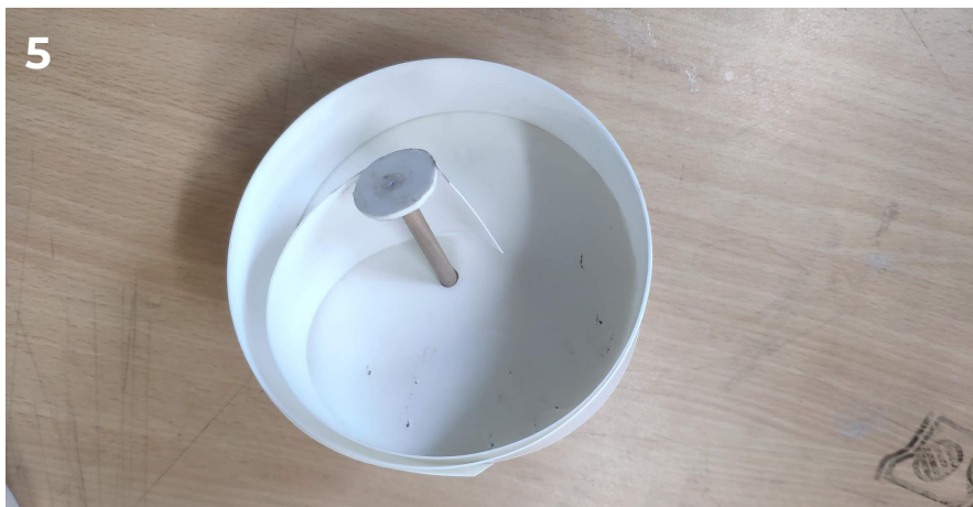
5 Rings are connected using a small wooden rod through them at the center.
