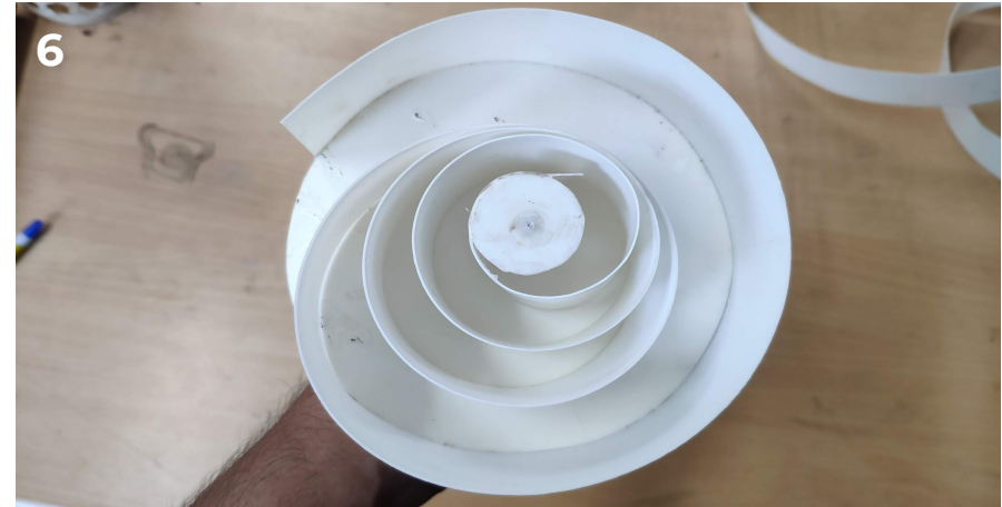
6 The spiral shape was formed, but it was not uniform because of its tensile strength. The surfaces tend to stack at one side of the circle.
