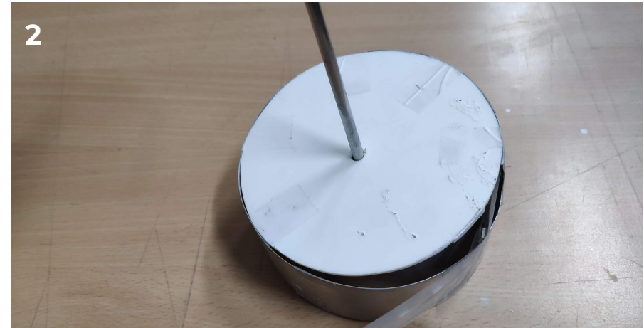
2 An aluminium rod is added, connected to the inner edge through the back cover.
