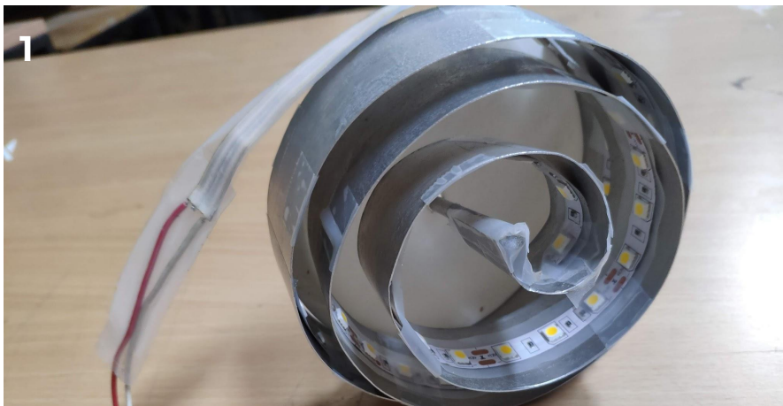
1 A back cover is added to direct the light in one direction.
