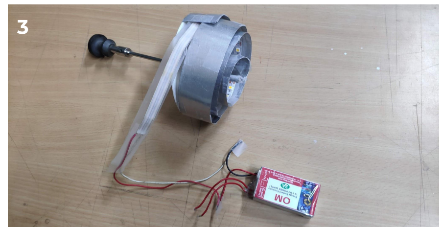
3 Aluminium rod is moved up and down to change the stage of the product from closed to expanded.
