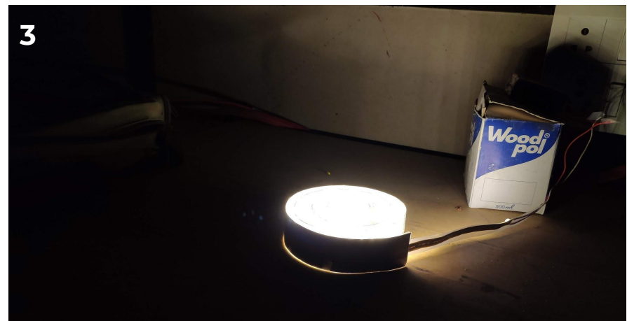
The LED strip light is fixed to the inner surface of the spiral and then tested.
