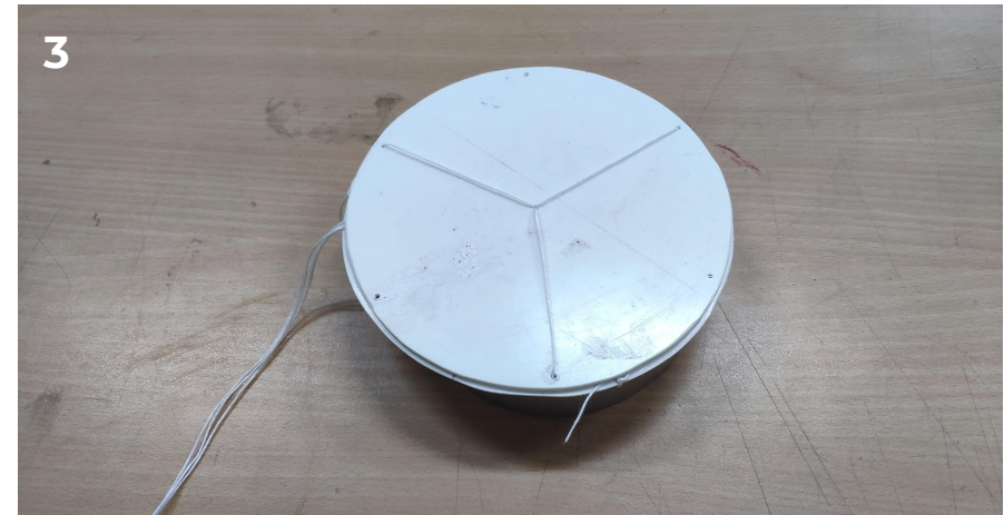
3 String from the circumference is taken back through the central hole to create a continuous connection for the mechanism.
