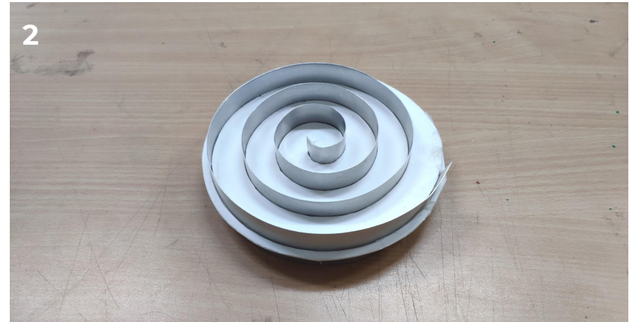
2 A strip 25 mm wide stainless steel is inserted inside the stencil to create a spiral shape.
