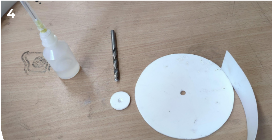
4 Another styrene strip is fixed on two rings, acting as a spiral's inner and outer end, using chloroform.
